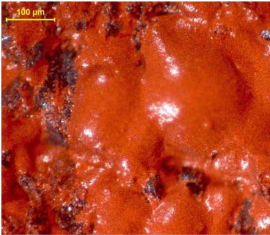
Figure 6: Example of observed filter cakes at the end of an experiment.
